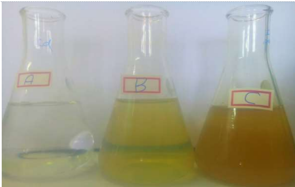
Figure-4: Green synthesis of Lead (Pb) nanoparticles A) PbNO_3 solution B) Cuminum cyminum seed extract and C) PbNP solution
